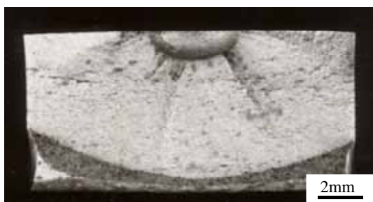
Fig. 9 疲労破面 p = 0.01368 N_f = 2143
